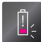
**Low battery alarm at 10.5V and low battery shutdown at 10.0V**
